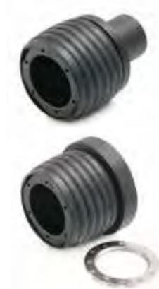
For the application list please check price list. Sparco collapsible hubs are cast iron made with a steel frame that collapse during impacts. This item absorbs kinetics energy avoiding transfer to the driver. The Sparco steering wheels are TÜV approved only if coupled with the Sparco hubs.
